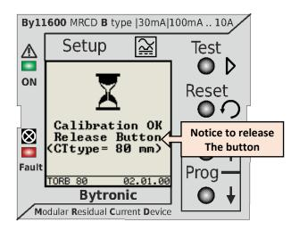
e) After giving the warning of 'Calibration OK' (and eventually releasing the button), the instrument performs a Reset and restarts in standard mode.
