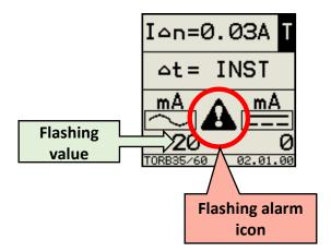
In the example it is assumed that the alarm threshold value of the alternating component (**ThAC Alarm**) has been set at a level lower than 66% with respect to the value of  $I_{\Delta n}$ .
