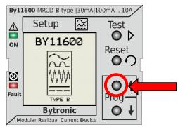
The 'UP' key has multiple functions, depending on the context of operation of the instrument.
