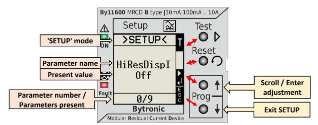
The right part of the display is related to the function of the adjacent keys, and each time in the 4 areas there are indications on the function of the relative key.
