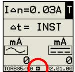
When the instrument is set up for protection against indirect contact ( $I_{\Delta n} = 0.03 \text{ A}$ ) no delay can be set. Delay  $\Delta t$  is adjustable only if  $I_{\Delta n} > 0.03 \text{ A}$
