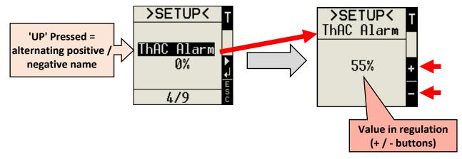
By adjusting the value to increase, the maximum value is reached and exceeded, the minimum is proposed again. Vice versa, by adjusting to decrease, once the minimum value is reached, the maximum is proposed again. Keeping the key pressed, the forward or backward will progressively faster. When the desired value has been reached, release the keys and wait.
