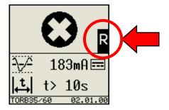
If it does not appear in the stored Fault or Alarm condition, it means that a Fault or Alarm condition is still present (not necessarily the initial one) and therefore Reset is not possible.
