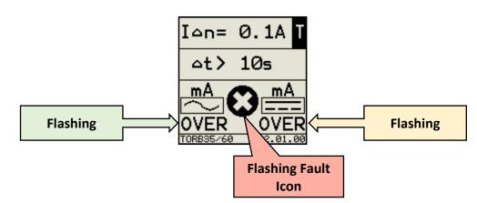
At the end, after  $\Delta t$  the Fault test trip will take place and, releasing the Test button, the negative R will appear in correspondence with the Reset button. See paragraph '<u>Reset</u>'.
