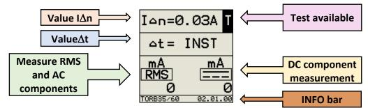
The displayed one is the page as per factory settings, in the absence of differential current. The RMS measurement of the current and its AC component alternates approximately every 3 seconds:
