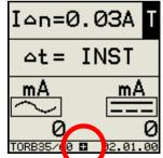
When the instrument is set up for protection against indirect contact ( $I_{\Delta n}$  = 0.03 A) no delay can be set. Delay  $\Delta t$  is adjustable only if  $I_{\Delta n} > 0.03$  A
