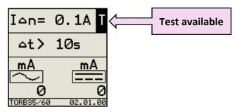
The test simulates the injection of maximum DC current to the measuring circuit. This injection of current causes an 'OVERFLOW' condition of the measurements.
