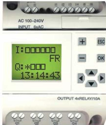
PLC AF-10MR-D ALIMENTAZIONE DA 10 Vdc A 28 Vdc
